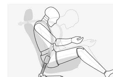
■ BMW restraint system for the driver and front passenger combines three-point safety belts, automatic safety-belt pretensioners, head restraints, and seat bolsters that help prevent occupants from sliding forward. This system helps provide optimum restraint in a collision.
