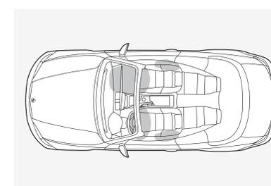
■ In a collision, BMW's SRS (supplemental restraint system) with advanced technology for the front airbags determines which airbags to deploy for optimal protection. The system also includes front-seat-mounted side-impact airbags.
