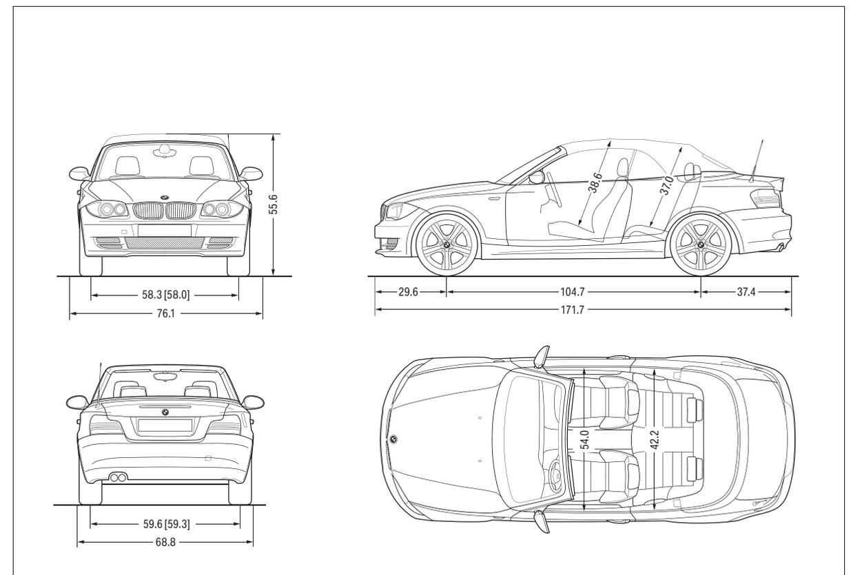
All dimensions are shown in inches, and apply to the 128i with standard wheels. Figures in [ ] refer to 135i.
