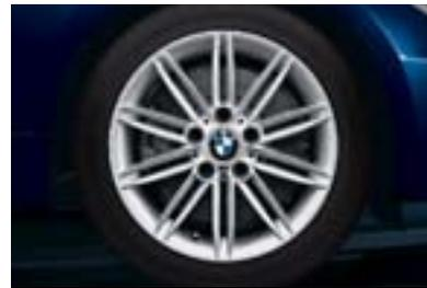
**BMW Double Spoke (Style 207 M) light alloy wheels and run-flat<sup>2</sup> performance tires.<sup>3</sup>** In front: 17 x 7.0 wheels and 205/50 tires; in back: 17 x 7.5 wheels and 225/45 tires. (128i M Sport Package)
