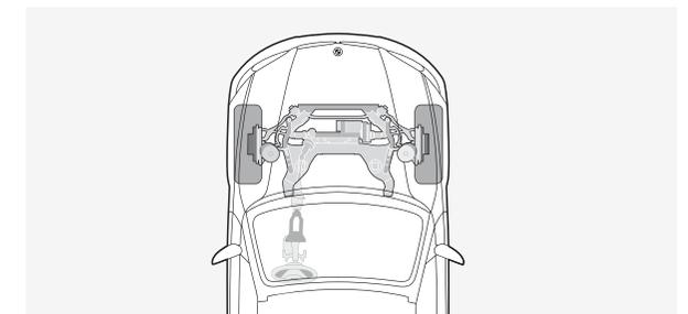
**Aluminum front suspension:** The 1 Series Convertible uses a lightweight, twin-joint tension strut suspension for maximum strength and minimum weight; hydro-mounts reduce vibration and noise. The overall result is noticeably athletic agility and responsive steering.
