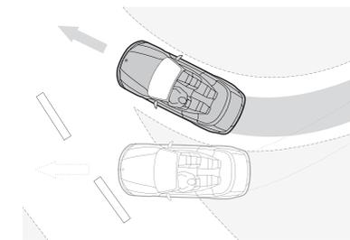
■ Dynamic Stability Control (DSC) with Dynamic Traction Control (DTC) features Brake Drying, Brake Stand-by, Brake Fade Compensation and Start-off Assistant. DSC is a braking control system that helps to stabilize a vehicle when it senses a loss of control. If the system senses over- or under-steer, it responds with counter-measures to help keep the vehicle under control.
