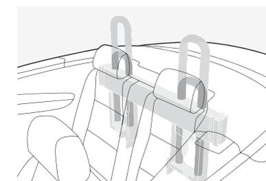
■ Rollover safety system consists of two steel rollbars behind the rear-seat headrests that are connected with a highly stable chassis crossbeam. The system includes a rollbar of high-strength tubular steel integrated into the frame of the windshield.
