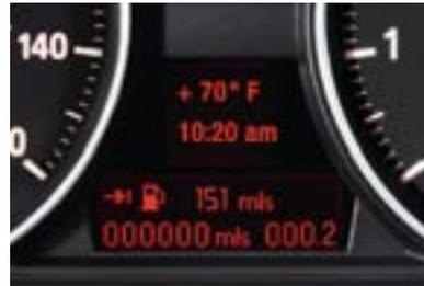
■ The **on-board computer** with Check Control provides feedback on the vehicle's operating status: oil level indicator and distance to next service appointment/oil change, as well as other detailed information, such as spark plug and micro-filter status. It also provides travel information: travel range on remaining fuel, external temperature, and more.
