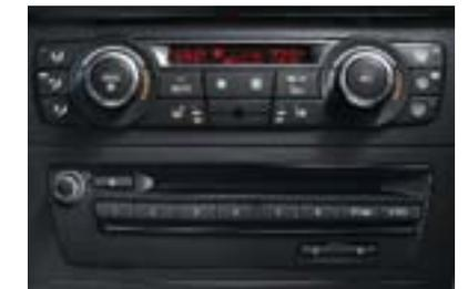
■ **Automatic climate control system** allows occupants to select a specific cabin temperature and choice of fan speeds, as well as automatic or manual airflow and recirculation. Convertible mode also reacts to exterior temperature and sunlight. The automatic recirculation control activates whenever certain air pollutants are detected. The system also includes defrost/demist and MAX A/C functions.
