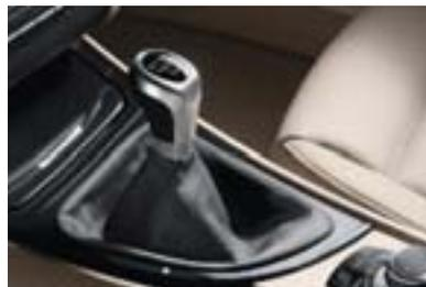
■ **6-speed manual transmission** delivers a precise, athletic feel. Its responsiveness is due, in part, to the enhanced synchronization of shifts from neutral to each gear. A shortened shift lever and throw add to the sporty feel of the gearbox. The sixth gear drops revs at highway speeds for smooth cruising.
