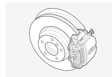
■ Massive, high-performance anti-lock disc brakes are ventilated at all four wheels for fade-resistant operation under hard use. (See page 65 for brake diameter sizes.)
