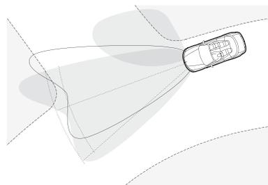
■ / □ Xenon Adaptive Headlights automatically swivel to follow the curves of the road. The system uses data from on-board sensors and the steering wheel angle to determine the car's direction, then adjusts the headlights accordingly. The system offers outstanding nighttime vision. (Standard on 135i; optional on 128i.)
