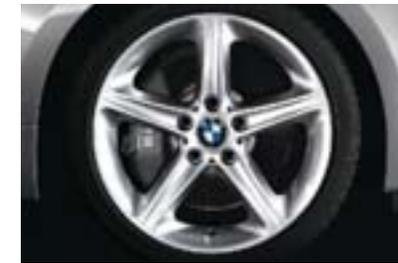
**High-performance disc brakes**, with inner ventilation and BMW painted on the calipers (6-piston calipers in front/2-piston calipers in the rear) measure 13.3" front/12.8" rear. Designed for high-performance driving, their large diameters help provide shorter braking distances and superior stopping ability.
