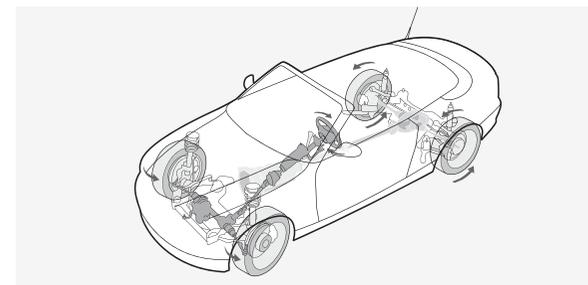
**Steering:** Torque steer is eliminated because steering and propulsion are not handled by the same pair of wheels. Steering force is evenly distributed; steering does not become harder; and steering-wheel angles are small. An added benefit: increased cornering speed.
