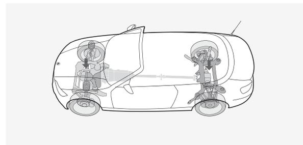
**Near-perfect 50/50 weight distribution:** The front and rear axles each carry almost exactly half of the car's weight. Balanced weight gives the new 1 Series Convertible neutral steering and outstanding directional stability. And with a sport-tuned suspension and DSC provided as standard, it remains stable in virtually all road conditions.
