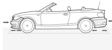
■ Impact-absorbing bumpers and compressible crush tubes front and rear help absorb the force of impact in collisions up to nine mph, minimizing damage to the vehicle's body and simplifying repairs. Only at higher impact speeds do structural supports begin to deform, dissipating impact energy to help protect occupants.
