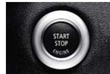
■ **Engine Start/Stop button** and remote key control the engine. First, insert the remote key into the starter switch slot. After the electronic identification system confirms that it is the correct remote key, you can start (or later, turn off) the engine by pressing the Start/Stop button. (Foot must be on brake; with manual transmission, clutch must also be depressed in order to start.)
