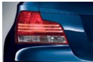
■ **Rear taillights** are made up of three separate high performance LED strips consisting of multiple rows of long-life LED indicators. The LEDs in each taillight unit provide greater illumination compared to the brightness provided by traditional bulbs.
