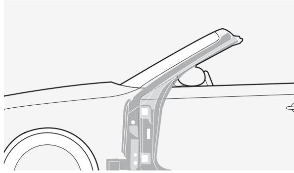
In the passenger compartment, the strengthened frame around the A-pillars and windshield acts as a rollover bar.
