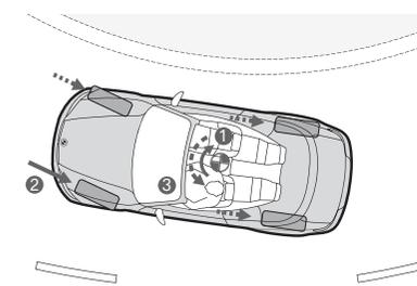
■ Cornering Brake Control increases vehicle stability by proportioning the braking force while turning. When you brake in a turn, the pressure comes off the rear wheels, which causes the vehicle to swerve inward (over-steer) (1). Cornering Brake Control counteracts this action by asymmetrically adjusting brake pressure (2), creating stabilizing counter-torque (3), independently of the ABS system.
