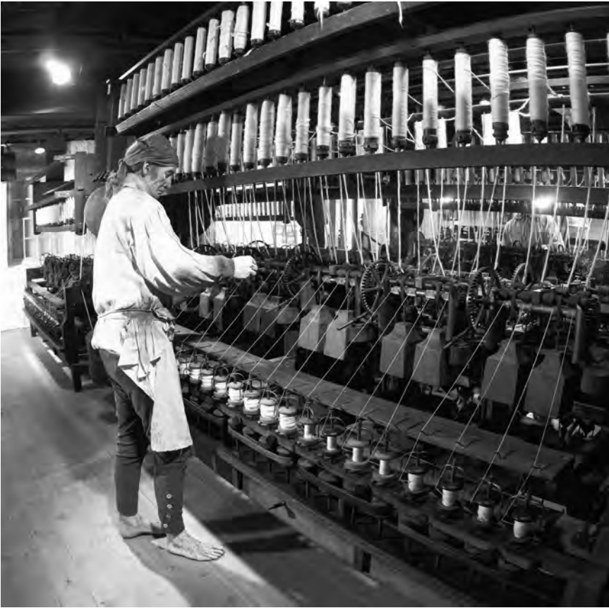
Figure 12.2 A water frame from Richard Arkwright's Cromford Mill, 1785.
