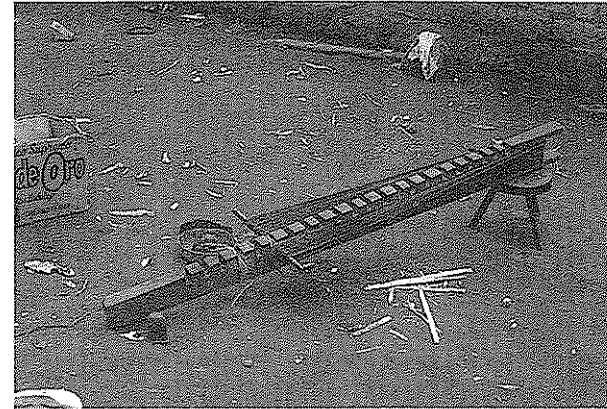
Fig 2.8. Warping frame, or homen , which requires mental transformation to visualize how the woven material will appear. A warp has already been wound. The left side of the threads will go to one end of the loom, say the top, while the threads on the right side will go to the other, the bottom.
