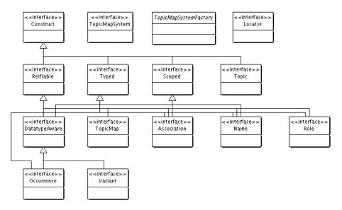
Fig. 1. Abbreviated UML class diagram for the "org.tmapi.core" package
