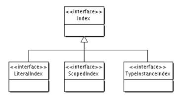
Fig. 2. Abbreviated UML class diagram for the "org.tmapi.index" package
